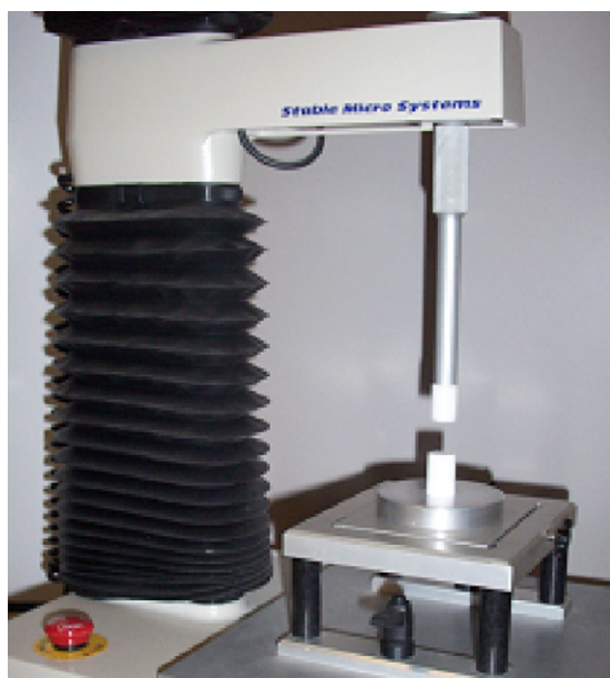
Fig. 2. Texture analyzer for the compression of powder plug for characterizing the crushing strength (degree of hardness).
